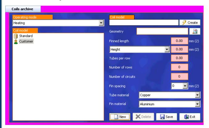
We insert the dimensions on the coils:
