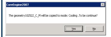
We can decide to Copy the geometry that we inserted in the Heating mode, into another modality like cooling. By clicking on the copy to mode:
