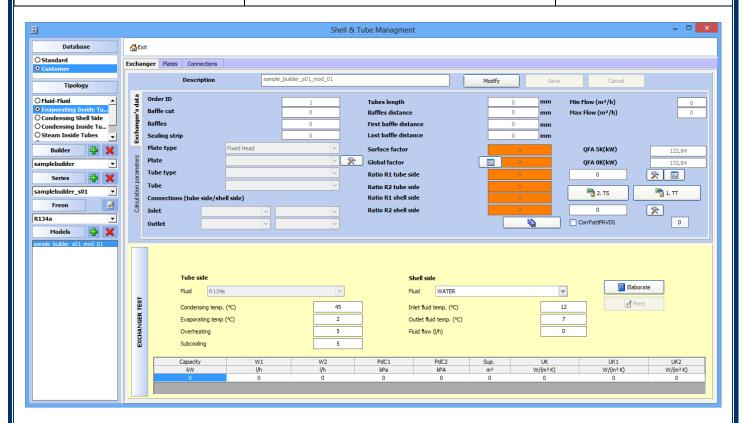
We note that we have to insert the plate model and the model of tube used by the heat exchanger:
