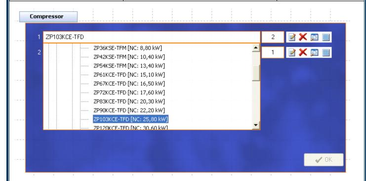
After selecting the compressor model wanted, we should set the number of compressors in tandem of the same type, by specifying its quantity in the field next to the model:
