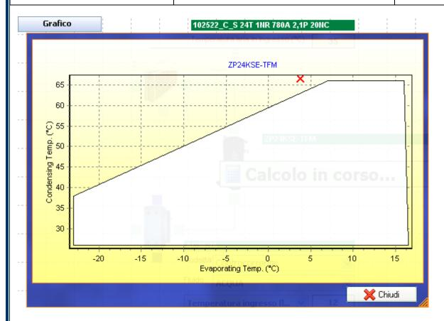
As we can notice, the compressor is condensing at 66,5 °C:
