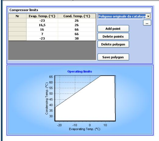
From the above figure, we can notice that in the evaporating range temperatures from 7  $^{\circ}$ C to 16  $^{\circ}$ C, the top condensing temperature allowed is è 66  $^{\circ}$ C. To insert a new envelope and not modify the default one, we click on list on the polygons like below:
