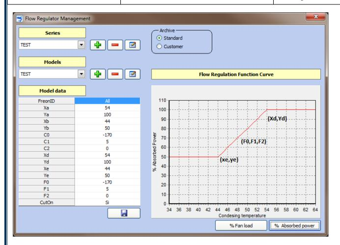
To insert a new series and a new regulator, it is possible to insert the data in the Customer Archive.
