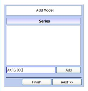
If it is necessary, like in this case, to add the series, write the name in the box below the list, and click on "Add":
