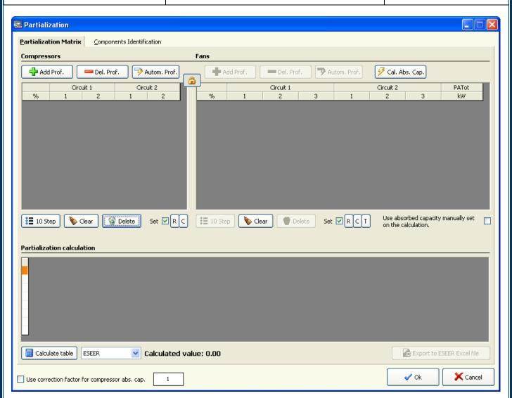
As you can see, this form is completely empty. It is divided into the Compressors partialization (left side) and the Fans partialization:
