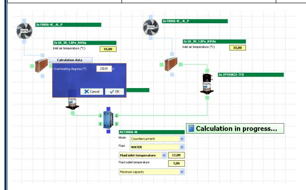
The first is to specify the overheating degrees on the condenser:
