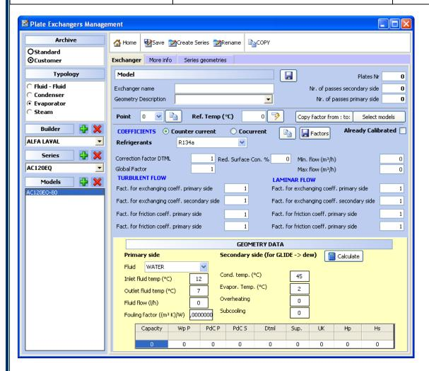
Now we have to insert the geometry of the heat exchanger. Click on the tab "Series Geometry" at the top. This is the window we get:
