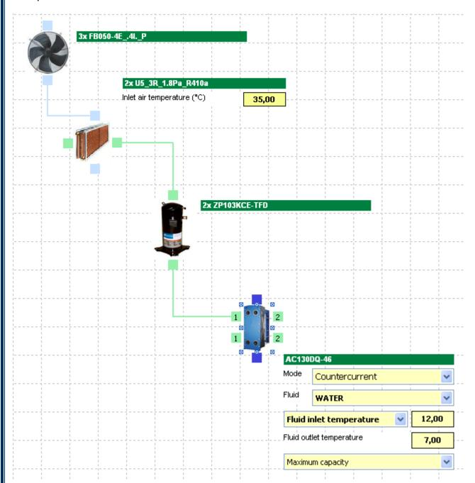
The green links are for the refrigerant circuit, the blue links are for the water circuit, and the grey links are for the air flow.
