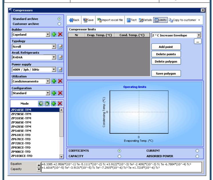
At this point, we click on "Add point" it is possible to insert the points of the new envelope, that will have to be inserted in anticlockwise and starting from the one on the lower left. Let's suppose they are the following:
