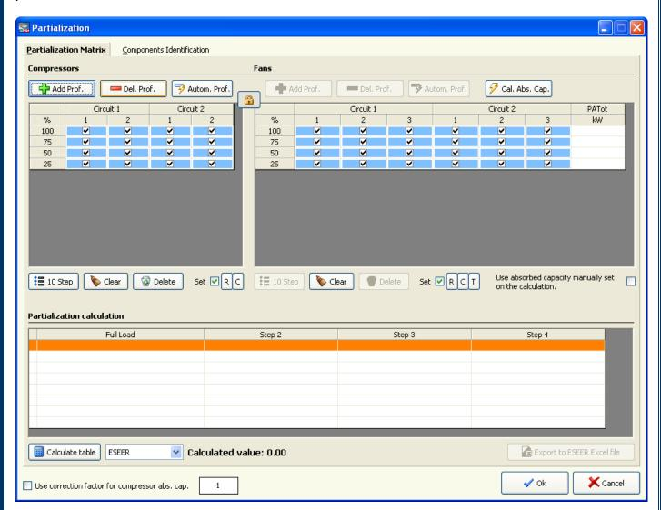
Each cell of the two grids represents the on/off state of the compressor or the fan:
