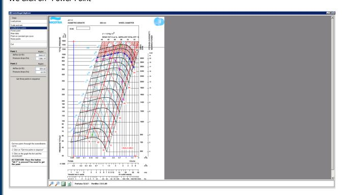
From the small guide we click on "Acquire" and we click on an intersection point between the constant efficiency curve and the power curve.
