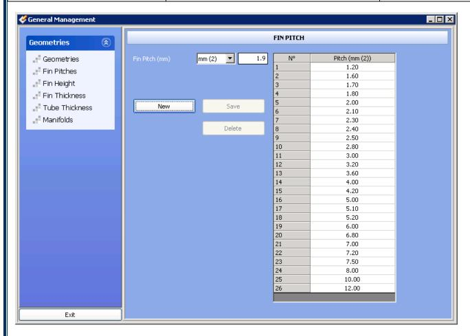
Suppose we want o add a fin pitch of 1.90 mm, so we can write the value "1.90" like in the figure, and click on "New" and you will see a message "The fin pitch will be added", we click on "Yes" to confirm.
