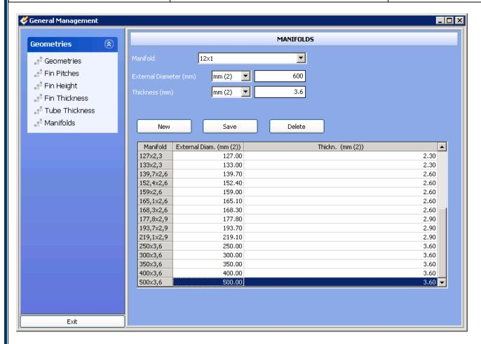
We click on Manifolds, and we insert the external diameter and the thickness, then we click on New. We click on "Yes"
