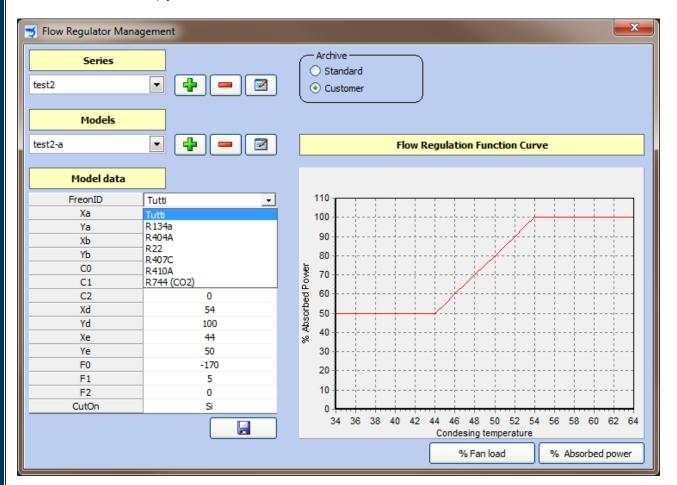
It is possible to simulate the fan shut down, choosing in the field "CutOn", YES or NO.
