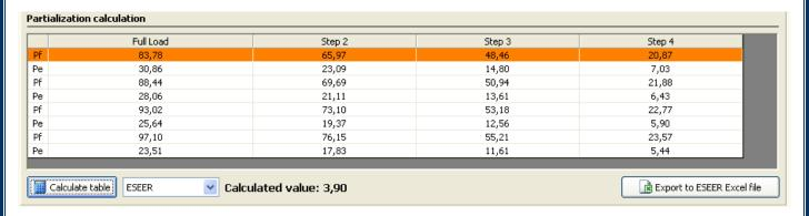
Please note that, as per ESEER calculation specifications, the unit at 100% condition is calculated with a fixed DeltaT on the fluid side, and on all the other conditions the unit is calculated with the resulting fluid flow.
