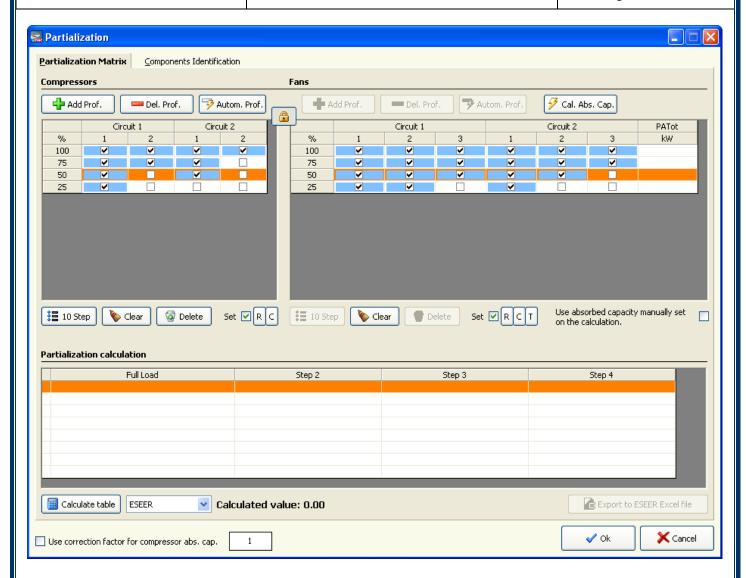
Look at the 50% row: in this case we set the first compressor of each circuit "on", but we can reproduce any other condition (like first circuit 100% and second circuit 0%):
