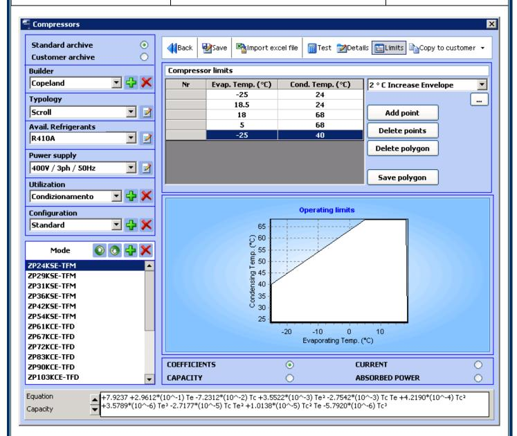
At this point, the compressor ZP24KSE-TFM is associated two envelopes, the default 1 and "Polygon 1", that has higher limits.
