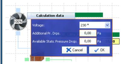
Additional pressure drops can be used to specify the pressure drop of the grid, and the Available static pressure drop is to specify a requested ESP.
