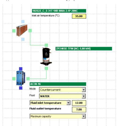
If we proceed with the calculation, after inserting all the requested data, the software will let us know that the compressor is working at condensing temperature outside the envelope:
